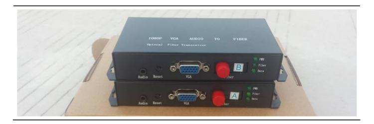
VGA to Fiber converter is designed to transmit VGA signals over optic fiber cable, with which we can transmit to 1-channel VGA signals and 1-channel Audio over one simplex optic fiber, Long Distance, Lossless, Non-compression, Real-time transmission. Well used in CCTV.
