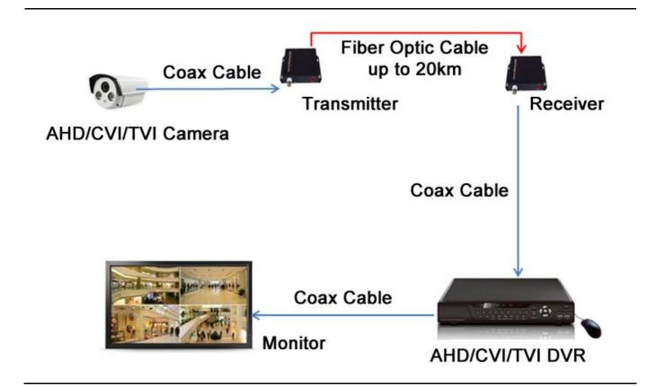
**1 channel TVI to Fiber Converter** is designed to transmit 1 channel TVI HD Videos over optic fiber cable, with which we can transmit 1-channel videos over one simplex optic fiber, Long Distance, Lossless, High definition, Non-compression, Real-time transmission. Well used in CCTV.
