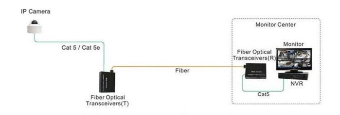
HK-0110-1V is a kind of intelligent, adaptive and fast Ethernet converter devices. It can implement data transmission between twisted pair electrical signals and optical signals which are the two types of network connection media. This kind of media converter can extend the transmission distance to 0.55 kilometers (multimode) or 20 kilometers (single mode). Using media converter is an economical solution to achieve long distance transmission base on current status.
